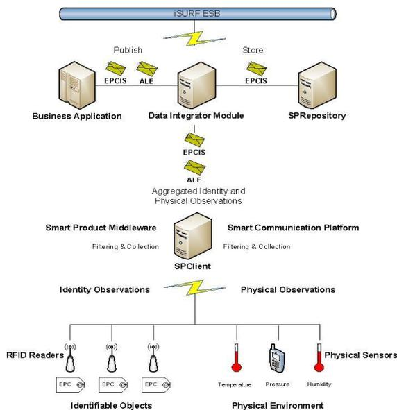
iSURF Smart Product Infrastructure (SPI), as shown in Figure 110, enables the tracking of items across supply chain historically in a near real-time fashion using RFID technology and delivery of RFID data to iSURF business applications and services to support their business processes seamlessly. The iSURF SPI is the lowest tier in the iSURF software stack and its primary function is the collection and delivery of data for use by higher level iSURF components.
