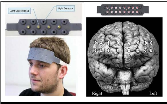
Figure 1. The fNIR Sensor (left) and Measurement Locations (right)<sup>12</sup>
