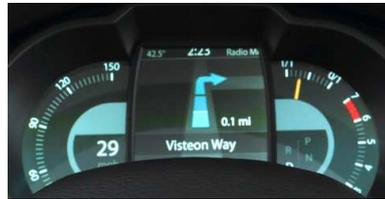
*Figure 1. Instrument cluster with fully reconfigurable display*
