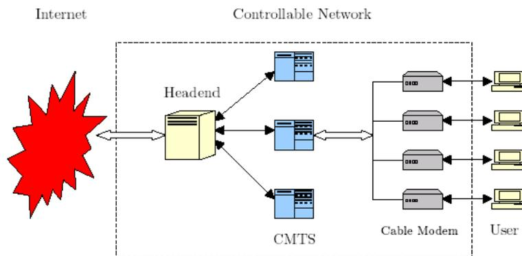
Figure 2. Network Diagram between End Users and Internet
