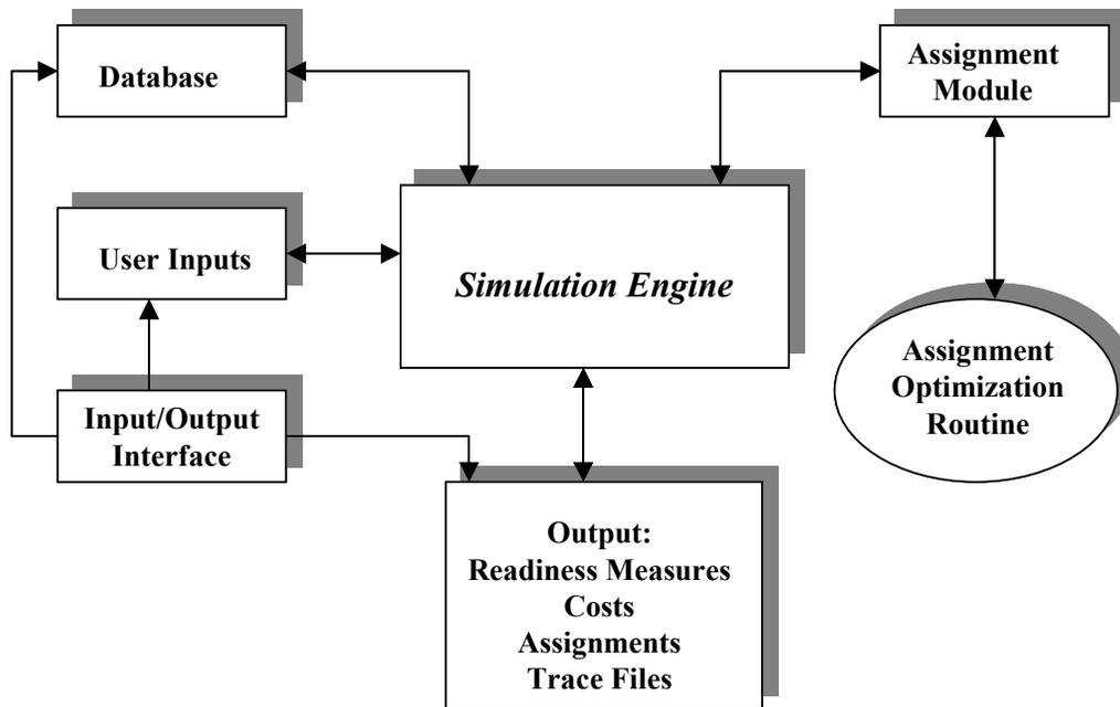
**Figure 1. Prototype Simulation Architecture**
