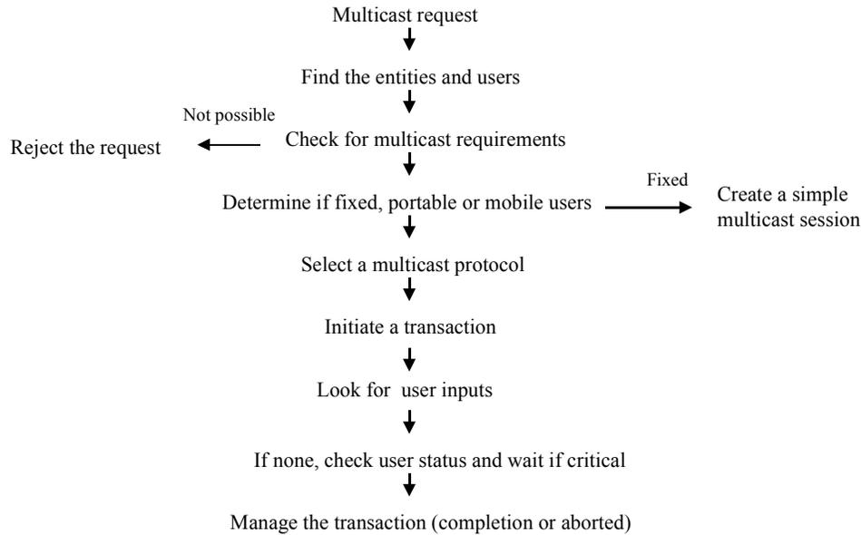
**Figure 4. A Step-by-Step Description of Multicast Process**
