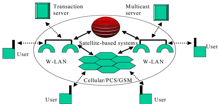
**Figure 2. Multicast Architecture for Mobile Services**
