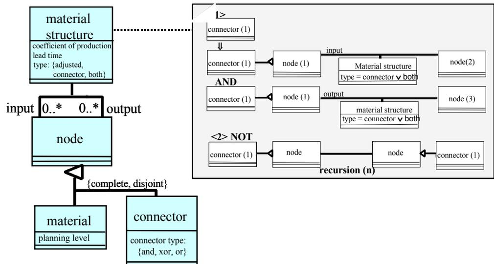
Figure 6. Class Diagram for Double-Coded Graph
