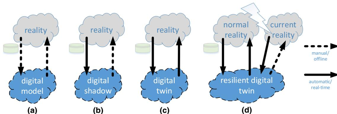
**Fig. 1** The difference between a digital model **a**, a digital shadow **b**, a digital twin **c**, and a resilient digital twin confronted with a disruption **d**. Visualization is based on (van der Aalst 2021a)
