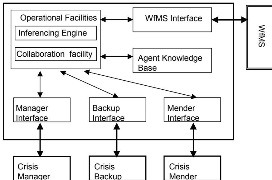
Figure 2. The Architecture of a Crisis Monitor
