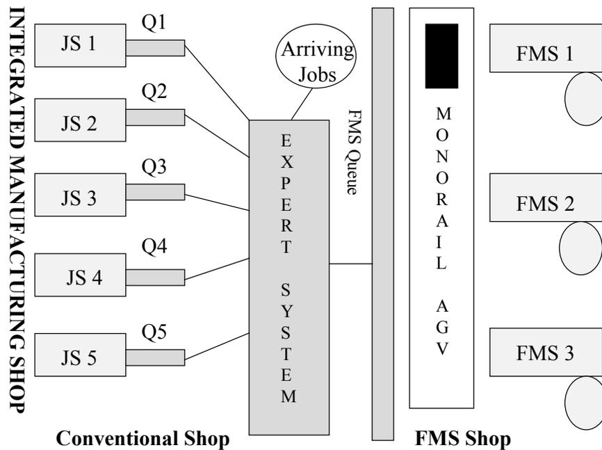
**Figure 1. Integrated Manufacturing Shop Model**
