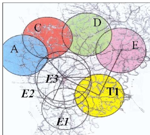
**Figure 2. Power Company's Wireless Expansion Plans. Legend: A: Repeater 1, service to approximately 800 residents. B: Repeater 2, 500 residents. C: Repeater 3, 500 residents. D: Repeater 4, 1,000 residents. E: Repeater 5, 1,000 residents. T1: 2-Hop Point-to-Point bridging link at 5.8Ghz.**
