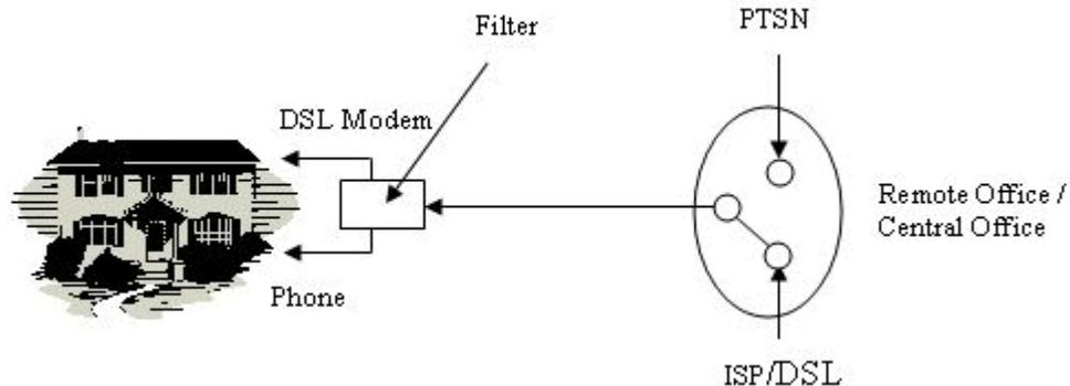
**Figure 1. xDSL solution to the Last Mile Problem, as adopted by the rural telephone company. PSTN: Publicly Switched Telephone Network. ISP: Internet Service Provider. DSL: Digital Subscriber Line.**
