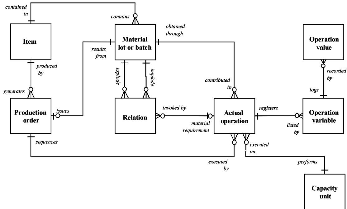
Figure 12. Tracking and Tracing Model
