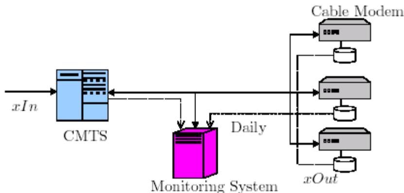
Figure 2. Monitoring of QoS level between CMTS and Cable Modems
