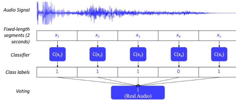
**Figure 5: Segmenting the data to feed into the classifier and using the max count as the final prediction**
