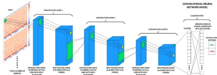
Figure 7: Architectural design of our CNN Model
