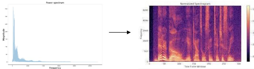
**Figure 4: Converting the spectrum into a spectrogram**
