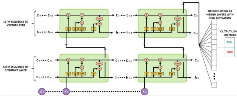
**Figure 8: Architectural design of our RNN – Long Short-Term Memory Model**
