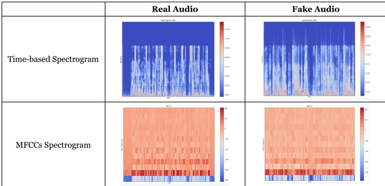
**Table 2: The time-based spectrogram and MFCCs spectrogram for a sample fake audio and real audio file**
