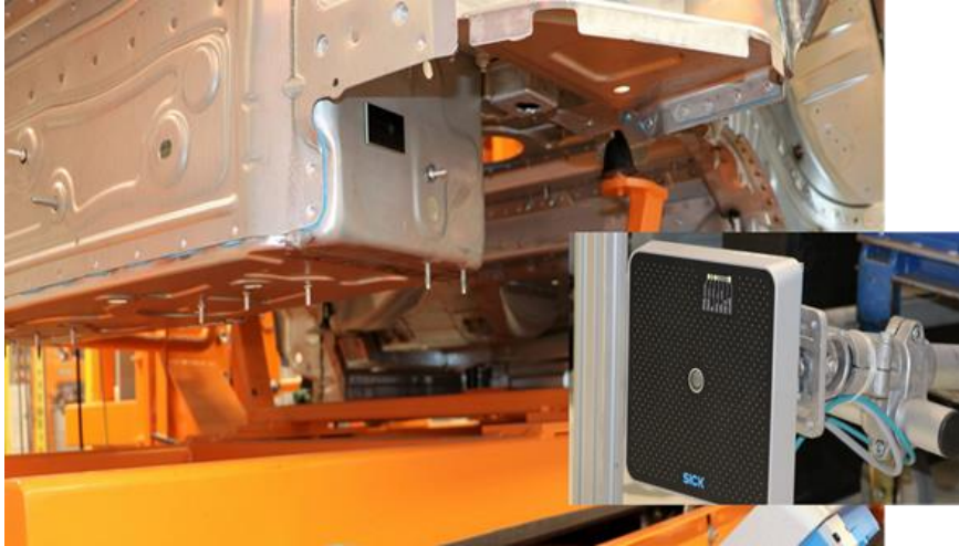
Figure 7. Order-Entry-Point: RFID-tag attached at the car body [AUDI]
