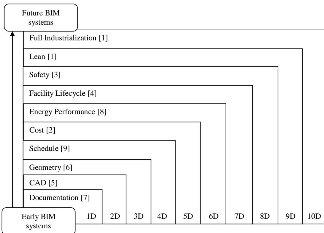
Figure 1: The dimensions of the BIM system
