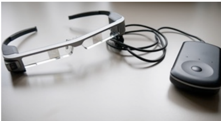
Figure 1. The Epson Moverio BT-300 HMD used for the Care Lenses and the Handheld Touch Controller (R)
