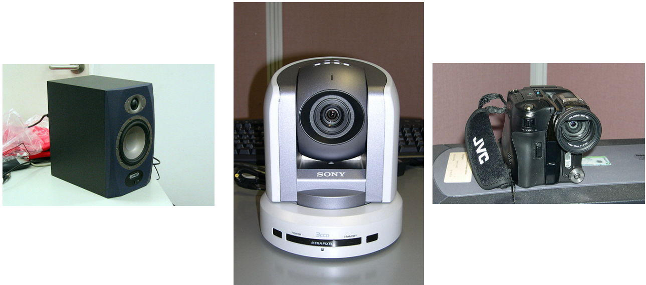
Figure 4. Some of the hardware choices in the videoconferencing setup Connected Cubicles . (a) Tannoy Reveal 5A amplified speakers, (b) Sony BRC-300P 3CCd tilt, pan, and zoom camera, and (c) JVC GR-X5AA 3CCD zoom camera.
