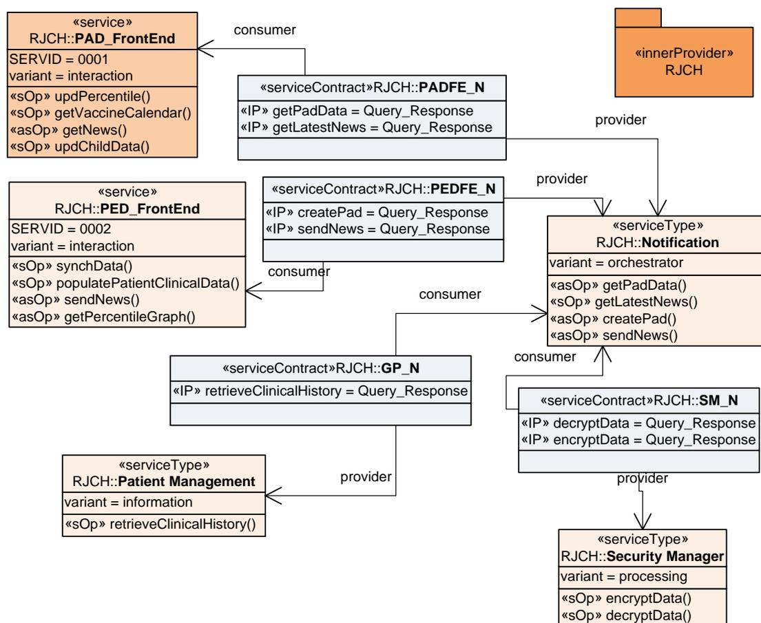
Fig. 3. Software architectural model at PIM level.
