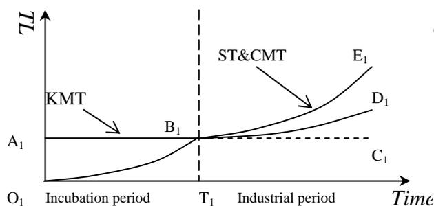
Figure 2. The synergetic development between system technology (ST), common module technology (CMT) and platform technology
