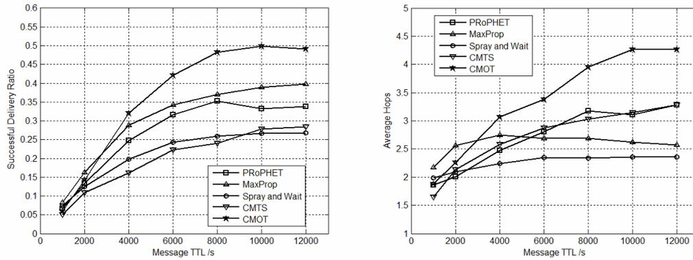
Fig. 10. Comparison of delivery ratio and average hops in different TTL
