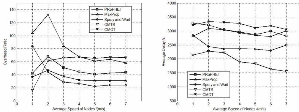
Fig. 9. Comparison of overhead ratio and average delay in different nodes' average speed
