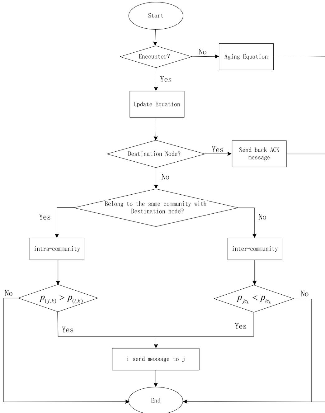
Fig. 2. The flow chart of message transmission process
