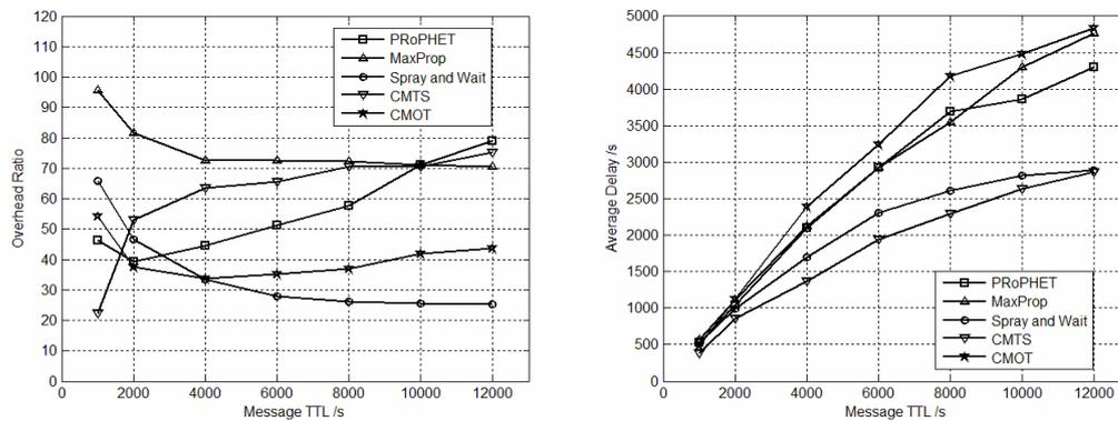
Fig. 11. Comparison of overhead ratio and average delay in different TTL
