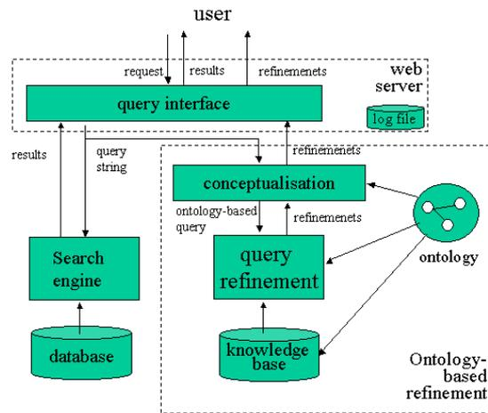
Figure 5: The integration of the logic-based refinement in a traditional information portal (a simplified model)
