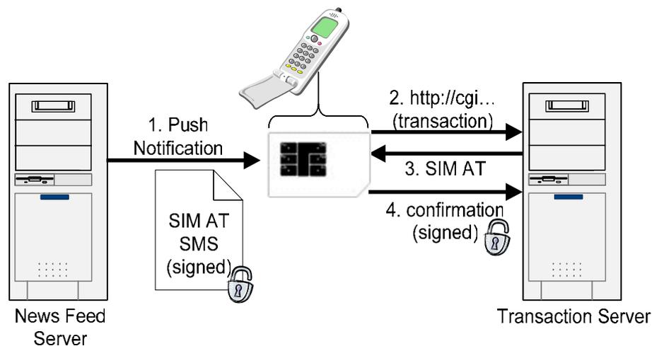
Figure 3. Notification and transaction system infrastructure (proposed)
