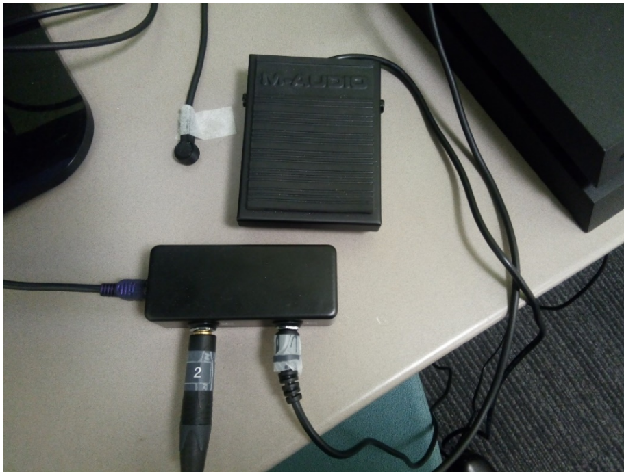
Figure 2: The DRT equipment (with stimulus at top left with white tape and foot pedal at top right).
