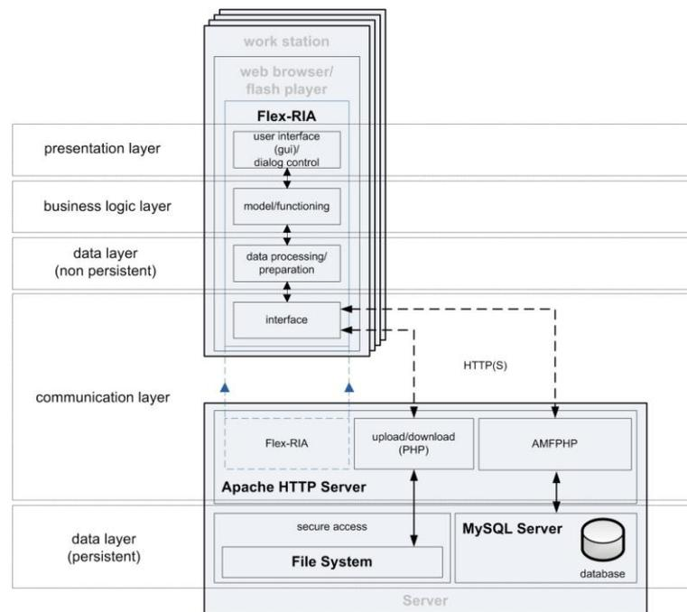
Figure 9. Architecture, Flex RIA and system environment
