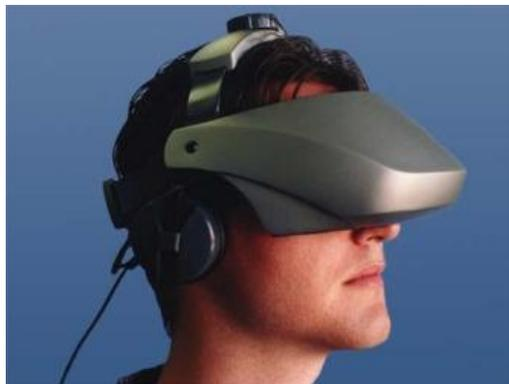
**Figure 1 Head Mounted Display**
