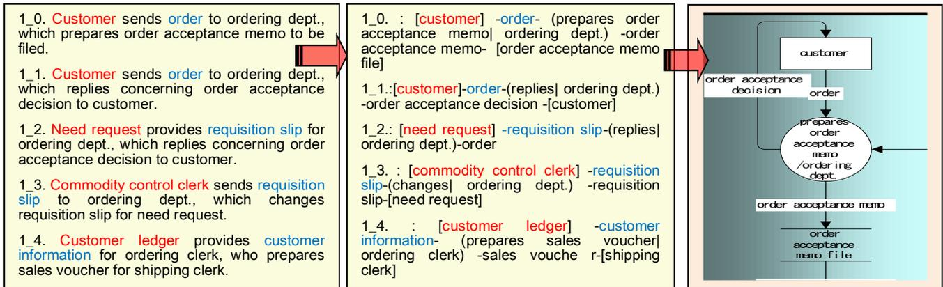
Figure 1. DFD generation (from NL to DFD via Structured inter-language)
