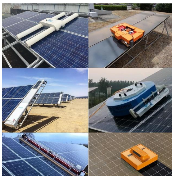
Source: Download from website ( https://image.baidu.com/ ). Figure 2: Two main categories of cleaning robot for solar panel.
