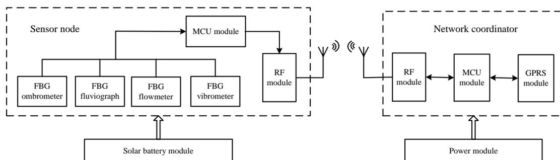
Figure 7. Hardware structure diagram of the monitoring system
