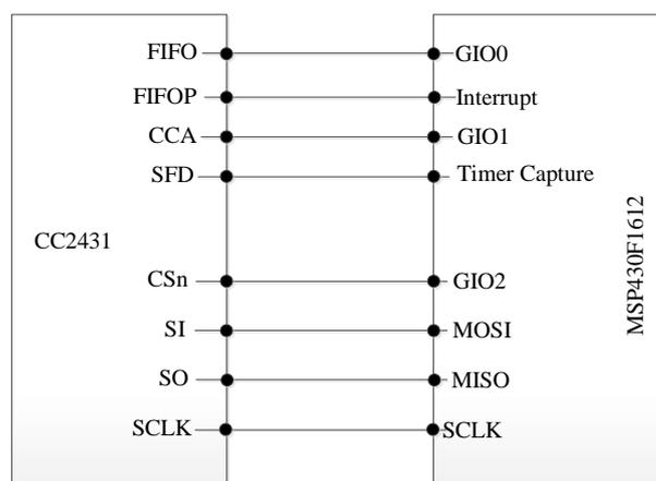
Figure 8. Interface circuit of RF module and MCU module
