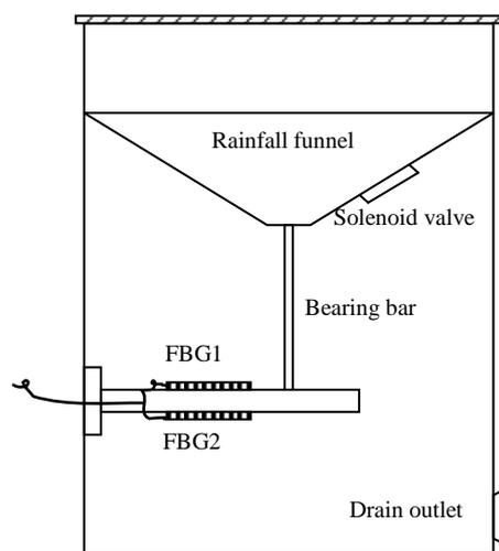
Figure 2. Structure diagram of FBG ombrometer
