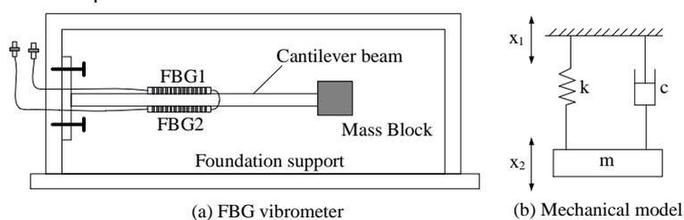
Figure 5. Schematic diagram of FBG vibrometer
