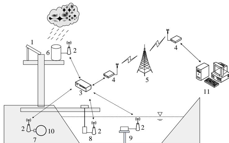
1: Solar power; 2: Sensor node; 3: Network coordinator; 4: GPRS module;
