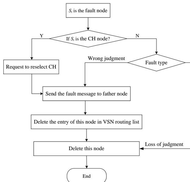
Figure 9. Fault node processing flow
