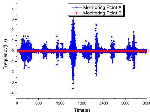
Figure 12. Frequency spectrum of pipeline subjected to flood scour
