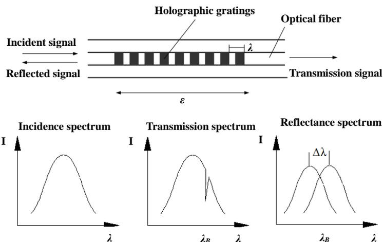
Figure. 1 Schematic diagram of FBG sensing principle
