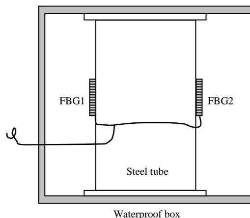
Figure 3. Diagrammatic drawing of FBG fluviograph
