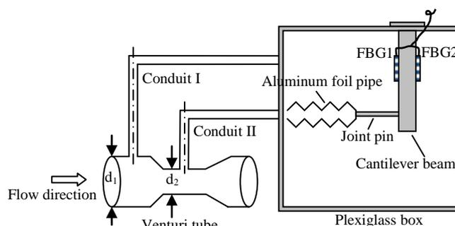
Figure 4. Schematic diagram of FBG flowmeter
