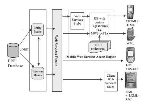
Figure 6: Architecture for mobile ERP system based on SOA concept
