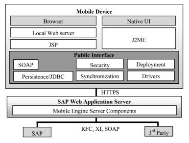
Figure 8: Software architecture of the SAP Mobile Infrastructure [cf. SAP04a]
