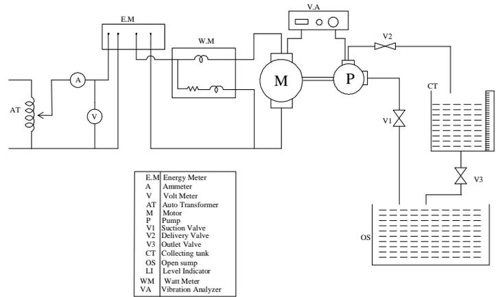
Figure 1 Schematic layout of the centrifugal pumping system
