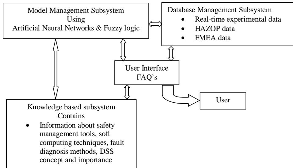
Fig. 2. Proposed DSS framework for safety management in centrifugal pumping system
