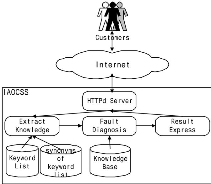
Fig 1: System Structure
