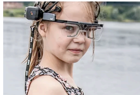
Figure 1. Tobii Glasses Eye Tracker with Emotiv Epoc+ EEG Headset[34]
