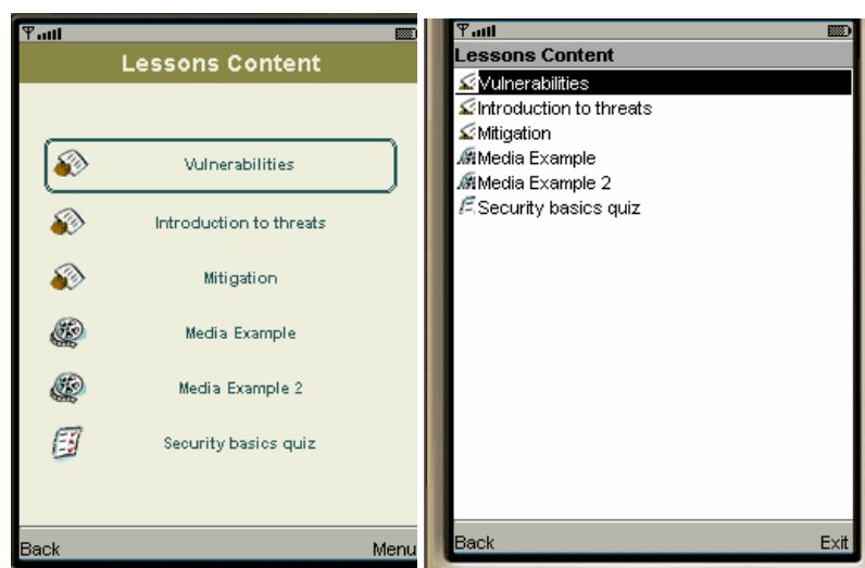
Figure 4: Generic J2ME user interface using J2ME Polish (left) and standard MIDP UI (right)
