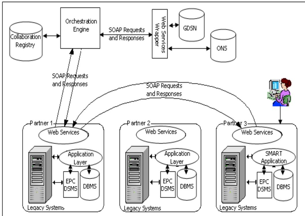
**Figure 2:** Schematic presentation of the scalable-distributed network architecture
