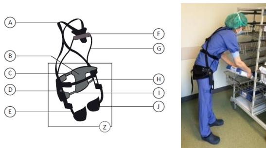
**Figure 1: Leavo exoskeleton**
