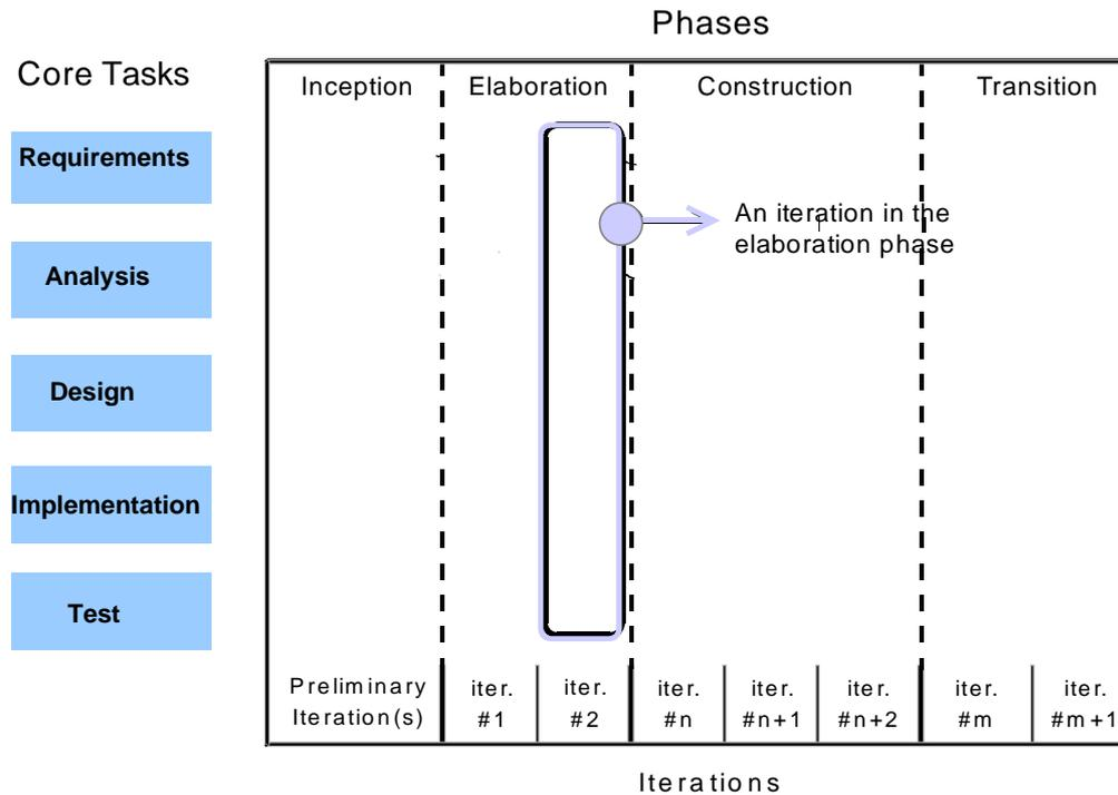
The phases correspond to the major milestones in the development of a software system. The Unified Process Model stresses that for each new version/release of the software, the process must be re-iterated. The phases coincide remarkably well with the information/knowledge handling process as proposed by Choo (Choo, 1998). The phases aim at the following milestones:
