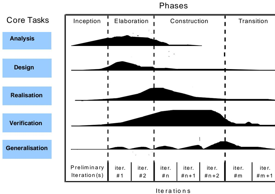
This picture illustrates, among other things, that modern software engineering processes use more energy for the verification than for the realisation of systems components, in particular when they reuse existing software components.
