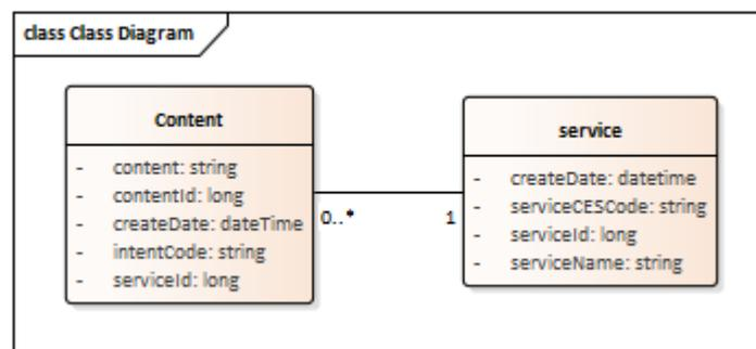
Figure 6 – Class diagram – services data structure
