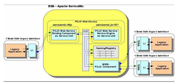
Figure 109 Legacy Adapters Overall Architecture
