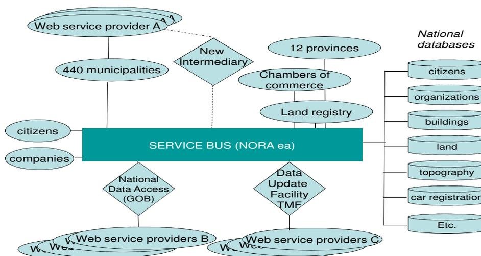
Figure 3: Municipality network with service bus, service clients, providers, and intermediaries
